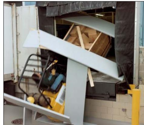
Vacant loading docks create a dangerous 4' drop-off for dock personnel and material handling equipment. The brutal reality of this dangerous drop-off is often recognized only after it is too late. Rite-Hite has a full line of barrier products to make your loading docks safer. Dok-Guardian Safety Barriers help meet the requirements of OSHA Regulation 1910.23 regarding "protection for wall openings and holes."
